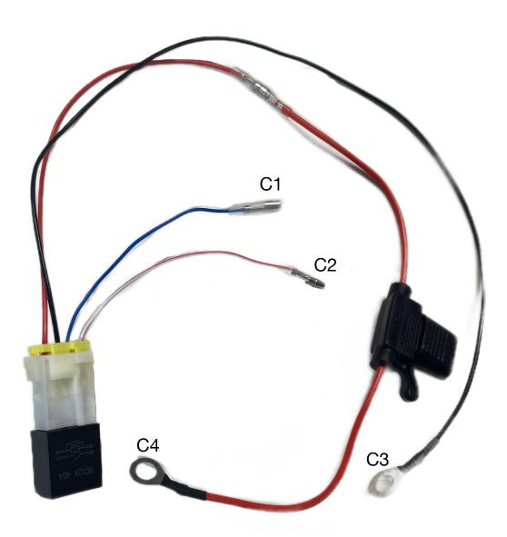
Connector 1 - Connect to desired ACC.
