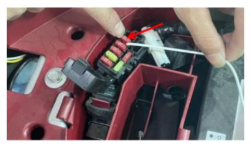
7. Pull the white wire to the position of the headlight, peel off the middle of the wiring harness(don't cut the copper wire inside), connect it with the red wire on the headlight, and complete the insulation measures, then connect the extra white wire to the red wire of the other headlight, start the vehicle after connecting, to check whether the headlights are electrified, as shown in figure:
