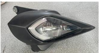
5.Install the new light in the same way as the removing of the original light, and fix it with the spare screws removed before (connect the plug-in of wiring harness on the light with the plug-in of wiring harness on the vehicle before installing the headlight), for the other side, replace the headlight as above Steps 2-4. As shown in figure:
