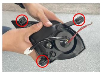
4. Install the outer decorative frame of the headlight, find the corresponding position, and directly lock it, as shown in the picture:
